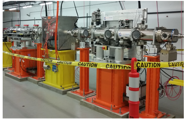
Figure 3: Both dechirper modules as installed in the SLAC LCLS. Between the two modules is a quadrupole magnet.
